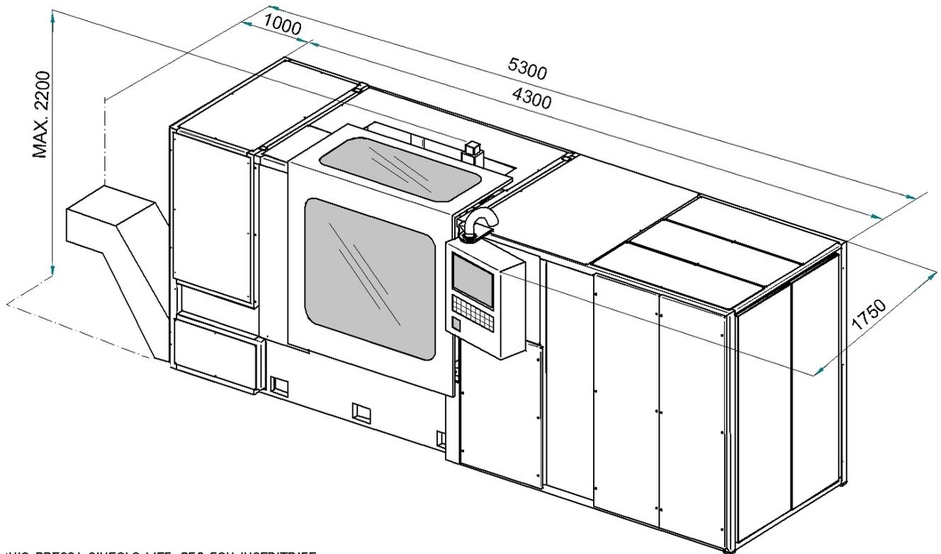
MACCHINA PRESSA SINGOLO MEC. 250 CON INSERITRICE
